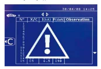
When the triangle sign is displayed, pressing key a second time definitively erases the contents of the report displayed on the screen. The triangle sign disappears from the screen after 3 seconds.
