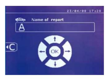
Recording a report allows to save the characteristics of a series of welding spots, and save them on the SD memory card, such that they can be transferred to any standard PC. GYS provides a software to read the SD card, and edit reports. This GYSPOT software is stored in the SD card, together with a copy of the user manual.
