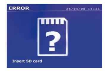
Switch off the machine, insert the SD card, and switch the machine ON again.
