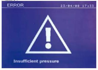
Pressing again on the button allows to force the execution of the welding spot, which will be performed with the air pressure available. If the actual measured clamping force is too low, then the machine will display the following message "Low Pressure".
