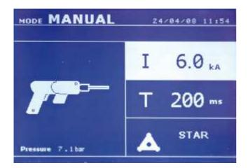
The single sided gun can be used in standard or manual mode. In normal mode, the single sided gun will be limited to steel sheets of thickness 1.5mm maximum.
