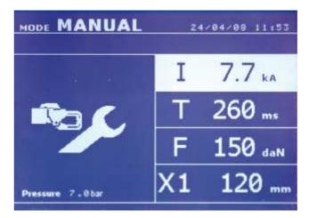
The key allows to switch from one tool to the next, and also allows to enter the clamp adjustment mode. The clamp adjustment mode allows to close the clamp and apply the selected electrode force, without delivery of any current. The clamp remains closed as long as the button on the clamp is pressed. This mode allows to check the alignment of the electrodes and the good positioning of the caps.
